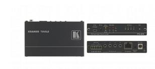
The FC-26 is a PoE-powered control gateway, capable of plug and play deployment over a customer Ethernet LAN for remote control of customer controlled devices via bidirectional RS-232 and IR control connections. Multiple control clients can be IP-connected to the FC-26 control gateway for concurrent control of two RS-232 and four IR controllable devices, such as AV scalers, video displays, audio amplifiers, and DVD players
